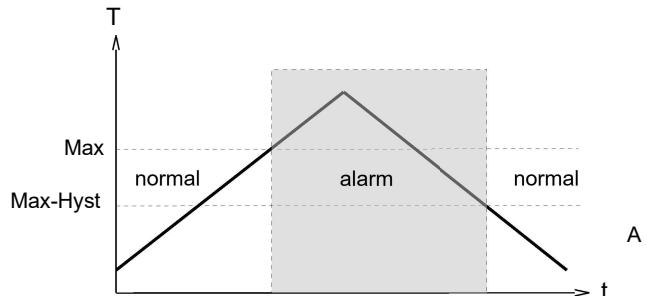
switchover delay time ( $t_{DS}$ ) can be applied to the switchover to the alarm state. Equally, one switch-back delay time ( $t_{DR}$ ) of several can be applied to switching back to the normal state.
