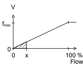
$f_{max}$  selectable in the range of up to 2000 Hz
