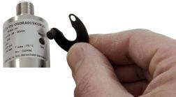
After the programming ("teaching"), the clip can either be left on the device, or removed to protect data.
