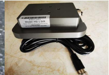
SVR is a non-contact method for measuring surface flow velocity in open channels. The SVR uses radar technology to measure the Doppler shift of electromagnetic waves reflected from the water surface. The Doppler shift is proportional to the water's surface velocity, and an calculate the velocity of water at various depths.
