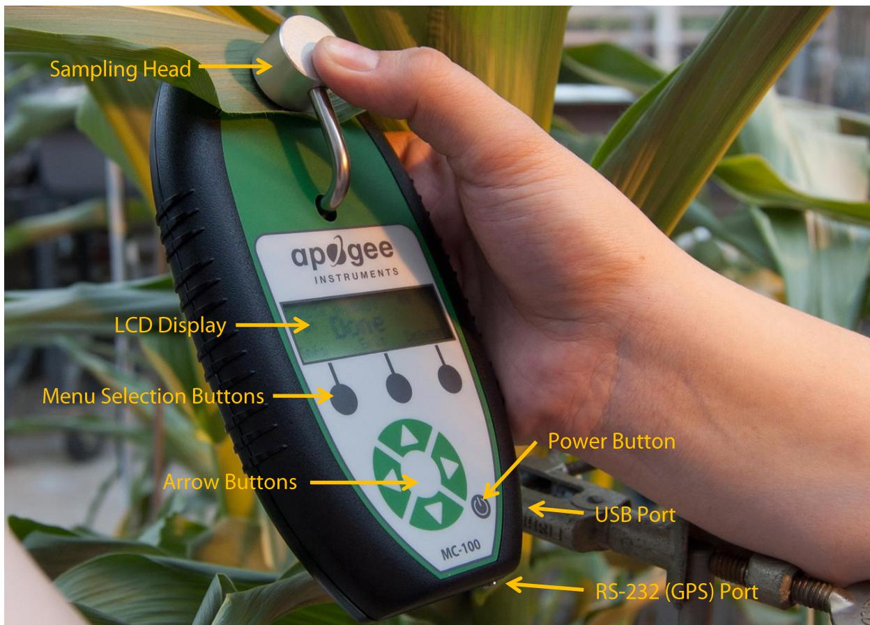
Press the power button to turn on the MC-100. After a few seconds the main menu screen appears. Program flow is organized into three menu groups. The selectable options are **Run** – used to set up and take measurements, **Data** – allows access and downloading of data files, and **System** – used to set up functional features of the meter and view system diagnostics.
