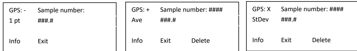
MC-100 with serial numbers 1521 and above have a "GPS:" icon in the upper left corner of the screen to indicate the status of the GPS signal and location logging ability. A “-” = GPS enable, no signal. A “+” = GPS enabled, signal acquired. An “X” = GPS disabled.
