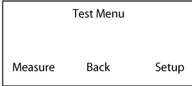
Select **Measure** to perform measurements with the MC-100 and **Setup** to make adjustments to data files, test types, and measurement parameters. Select **Back** to return to the main menu.
