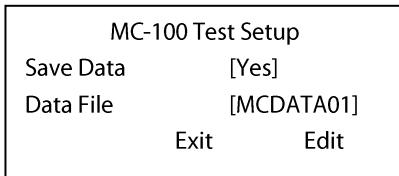
The user can choose to save a data file to memory in addition to naming the file. Select **Edit** to highlight the **Save Data** option. Pressing the up and down arrows will toggle between **Yes** and **No**.
