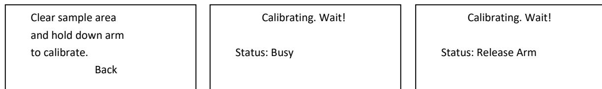
The MC-100 requires a calibration when taking the first measurement after powering on the unit. **Calibration is not required between measurements.** Verify the sample chamber's optical path is clear and hold down the measuring arm until the **Release Arm** message is displayed.
